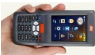
DAP Technologies introduced the M1000 handheld computer that is hardly larger than a standard mobile phone, but has voice capability and a barcode scanner or imager, making it suitable for inventory control, picking and packing and other advanced scanning applications. Powered by a 624MHz Marvell PXA310 processor
