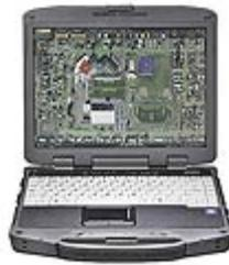
Now equipped with a 2.2/2.9GHz Intel Core i7-2655LE processor and ancillary circuitry, the General Dynamics Itronix flagship GD8200 should be substantially more powerful than its predecessor, while retaining full backward compatibility and its 8-hour battery life rating. Graphics performance is improved and additionally benefits from DynaVue II technology. The IP65-rated GD8200 also supports numerous wireless standards including 4G LTE. [See the [GD-Itronix GD8200](#)]
