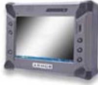
DRS Tactical announced the release of the DRS ARMOR X7 rugged tablet computer, which will complement the company's larger X10 rugged tablets. The Intel Atom N450-based X7 has a 7-inch WSVGA display with auto-sensing dual input (active digitizer and resistive touch), is exceptionally rugged (6-foot drop, IP65, -4 to 140F), weighs under three pounds, and offers excellent configuration and customization potential via expansion bays and "FlexSpace" interfacing [Read about the [DRS ARMOR X7](#)]
