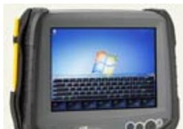
DAP Technologies added the M9000 line to its growing lineup of rugged handhelds, vehicle-mounts and tablets. The M9010 tablet is a significant tech update to the M8910, using an Intel E660T Atom processor to run either Windows CE 6.0 or Windows Embedded Standard 7. There's a
