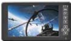
Taiwanese industrial display technology and rugged solutions provider Winmate introduced a minimalist rugged device geared towards providing GPS information and computing power for military and similar deployments in the smallest possible package. The Atom Z530-powered tablet has a sunlight-readable 7-inch resistive touch display and weighs less than two pounds. [See description and specs of the [Winmate 7-inch rugged tablet PC](#)]
