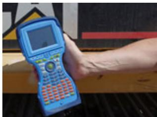
There's rugged, and then there's ultra-rugged, nearly indestructible and fully waterproof. That would describe the highly customizable Hydrus handheld from Two Technologies. It's a 2.5-pound Marvell PXA270/Windows CE-powered handheld with a large 55-key keypad, a 5-megapixel imager/scanner with laser auto-focus and illuminators, 40 hour battery life, and yes, we even tested it underwater [See full review of the [Two Technologies Hydrus](#) and see [YouTube video of the Hydrus underwater](#)]
