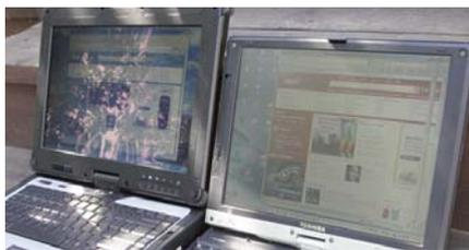
Overall, Samwell's outdoor-viewable technology is impressive. At times you have to position the notebook to stay clear of reflections, but there is always enough contrast and brightness to use the computer outdoors, under any lighting conditions.
