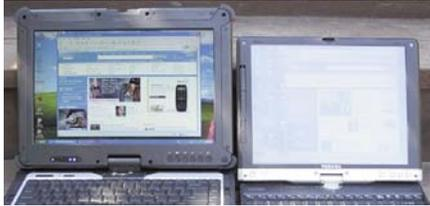
In the picture below, the two machines are in the same location, but the image was taken from an angle. The SR858's display remains very readable with just a bit of reflection from its surroundings. The older display's matte surface diffuses the light so much that the screen becomes unreadable.
