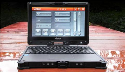
The screen offers Getac's capacitive 5-point multitouch technology, and there's also an optional active digitizer with a small, very precise pen that does not need a battery.
