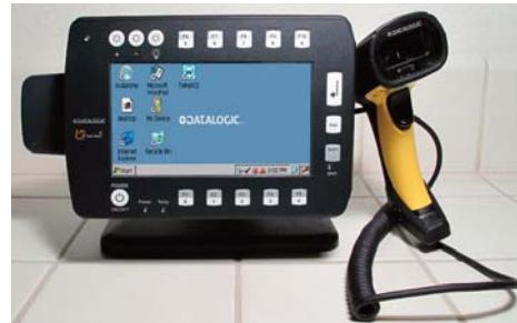
compact external keyboards with both ABCD and QWERTY layouts. Input can also be via touch in custom applications, or via onscreen keyboard. The R7 comes with the standard Windows CE pop-up keyboard and also with the significantly more extensive My-T-Soft keyboard/input panel.
