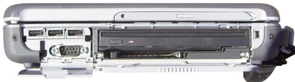
but not just any plastic. This is TPU-- Thermal Plastic Urethane, the stuff they use to make rollerblade wheels from. Itronix used this material for three reasons. It makes the unit feel cooler to the touch in places where it heats up. It is more conducive to RF performance. And it is nearly indestructible.
