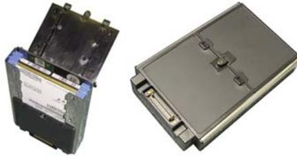
around the axis, to warm up the grease. The pictures below show the hard drive's protective case, open on the left so you can see the blue shock mounting sub-frame, and closed on the right. A very clean design.
