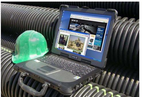
L2400 processor with a 667 frontside bus and 2MB of L2 cache. It moves smartly and the processor is an excellent compromise between all-out performance and decent battery life. Standard memory is 512MB of DDR2 RAM, and that is expandable to 2GB in a total of two slots. The standard graphics controller is an Intel GMA950. The machine is optionally available with an ATI M54 graphics chip with
